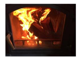
**Step 4** Add more logs as required to build a really good base to the fire, then reduce air flow via controls, to suit requirements.
